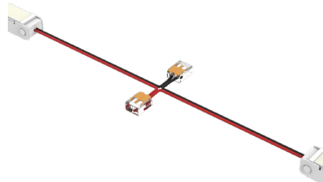
Detail B Dry Splice Connection (Connectors by Others)
